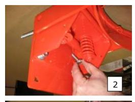
Adjust "Flush-Mount" back plate so that it matches the rim mounting pattern on your backboard. Using a 9/16" socket and standard screwdriver, tighten hex nuts to secure the "Flush-Mount" plate in place being sure to keep it square. (Use 30 lbs. torque)
